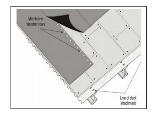
An air barrier is also recommended for mechanically attached systems to help reduce billowing from internal air pressure. Air barriers need to be taped where breaks occur.
